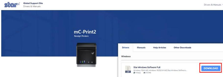
3. Connect printer mC-Print2/3 to PC by USB Cable then open Printer Utility and select which printer you want to setting then click next
