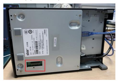
2. The factory default setting of dip switch will be same as below picture of each model, so if you want to disable auto cutter in case of SP747 model, should be change dip switch 1 bit 2 from OFF to ON
