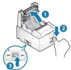
• When the LED (blue/red) flashes alternately 4, release the Feed button 5.
