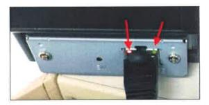
7. **For Thermal Printers:** Confirm with a self-test page that the printer was able to reset the NIC card properly. To perform a self-test page, turn off the printer then hold the "feed" button on the front of the printer while turning the printer on. Let go of the "feed" button when the printer starts to print. It will print out two pages.
