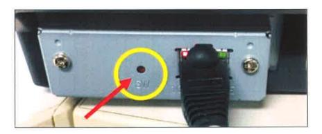
4. With a small screwdriver or pin, you will press the "SW" button until both the NIC LED lights start blinking, then let go of the "SW" button. Both NIC LED lights will be solid.
